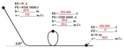
The roller coaster begins with 450 000 J of mechanical energy (all in the form of PE). It conserves this energy; so the sum of the KE + PE is 450 000 J at all positions. If KE is known, PE can be calculated (and vice versa). The speeds (**v**) are related to the KE values by the equation  $KE = \frac{1}{2} \cdot \mathbf{m} \cdot \mathbf{v}^2$ . The heights (**h**) are related to the PE values by the equation  $PE = \mathbf{m} \cdot \mathbf{g} \cdot \mathbf{h}$ .
