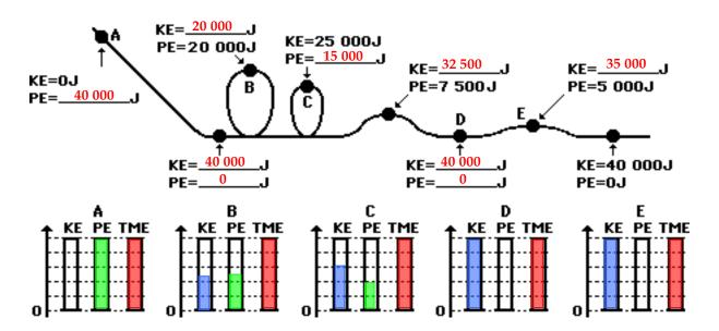
11. Use the law of conservation of energy (assume no friction) to fill in the blanks at the various marked positions for a 1000-kg roller coaster car.
