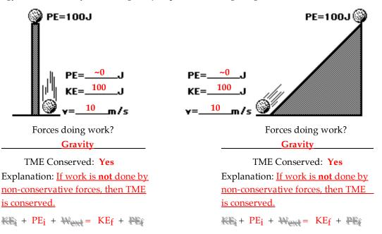
2. Use the work-energy relationship to fill in the blanks for the following system (m=2 kg). Neglect frictional forces. Finally, darken in the bars of the bar chart in order to demonstrate the amount of kinetic energy (KE), potential energy (PE) and total mechanical energy (TME).
